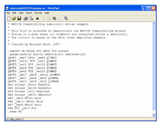
The HSPICE design can be used like any ADS component. If you have pins, you can connect it with ADS hierarchy. If a top level design was designated, it will have pins. If a subcircuit was chosen, it will have appropriate inputs.
